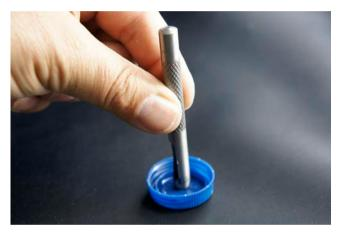
Fig. 51: Example of method for punching holes in bottle caps
